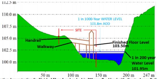
Section demonstrating the Finished Floor Level and a 1 in 200 year flood level with climate change Both in AOD.
