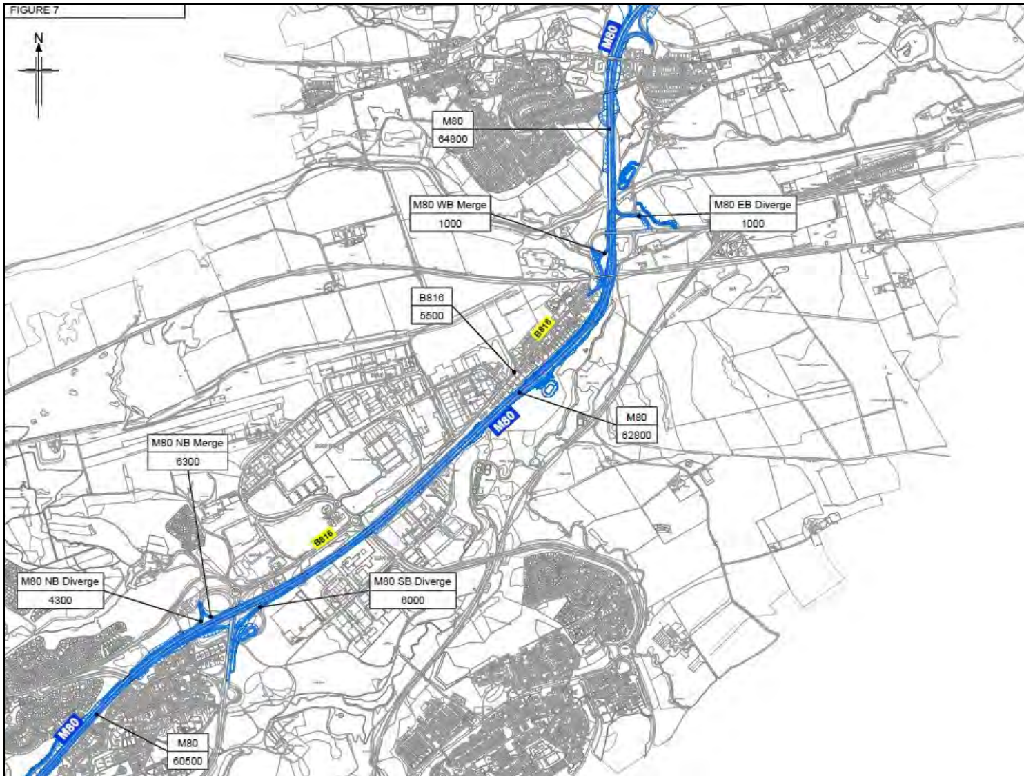
Figure 7: Existing AADT Flow levels
