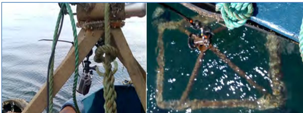
Image A.1. Mobile frame used for drop down video survey
