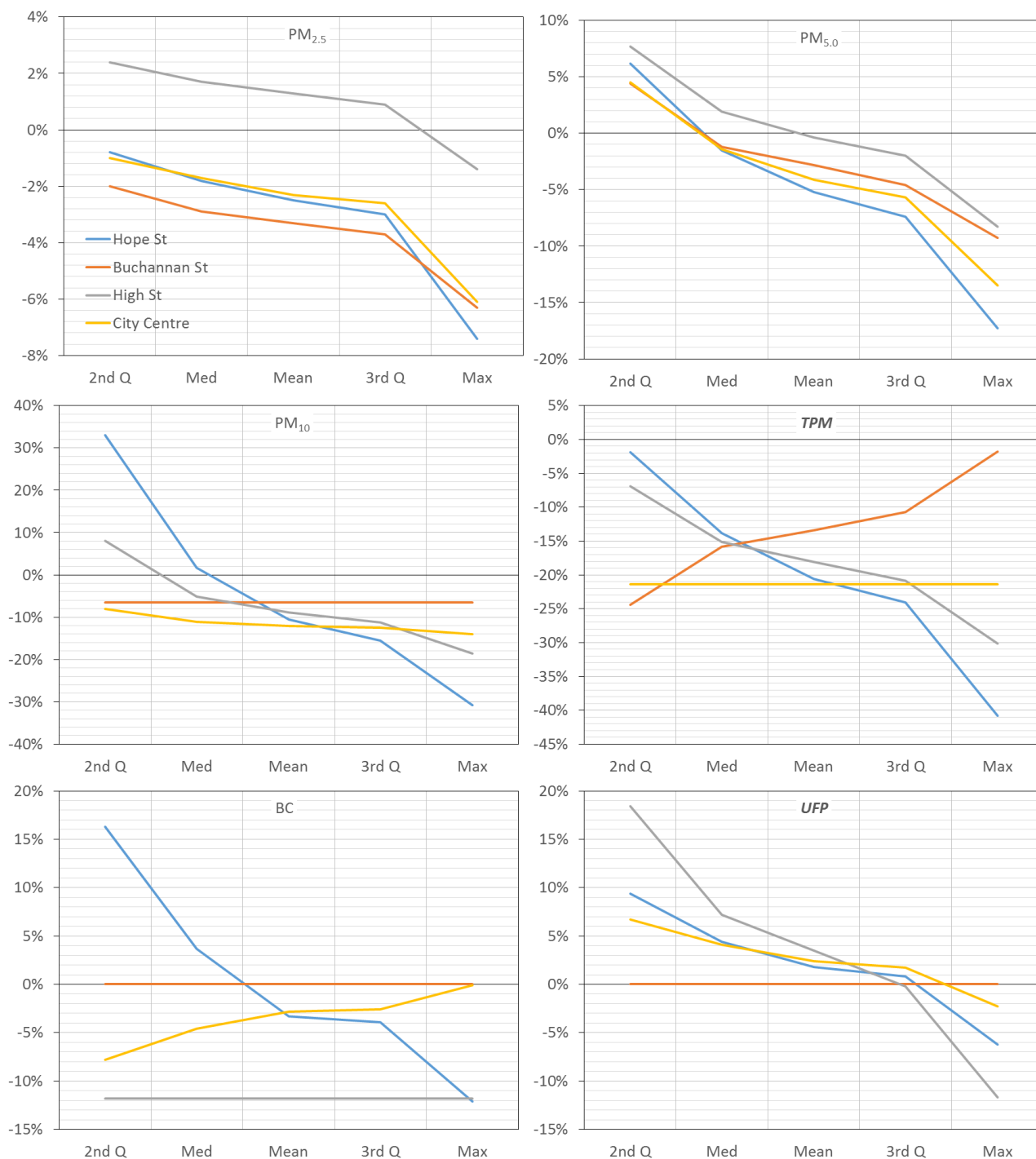
Figure L7 Percentage Difference in Measured 1-minute Average PM_{2.5} , PM_{5.0} , PM_{10} , TPM, BC and UFP Concentrations at 0.80 m and 1.68 m
