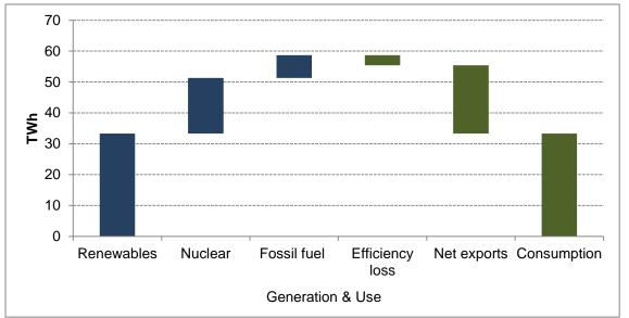
Figure 9: Electricity Generation and Use in 2020 (TIMES model results), (Electricity storage technologies are not in the above as they are deployed further down the supply chain)
