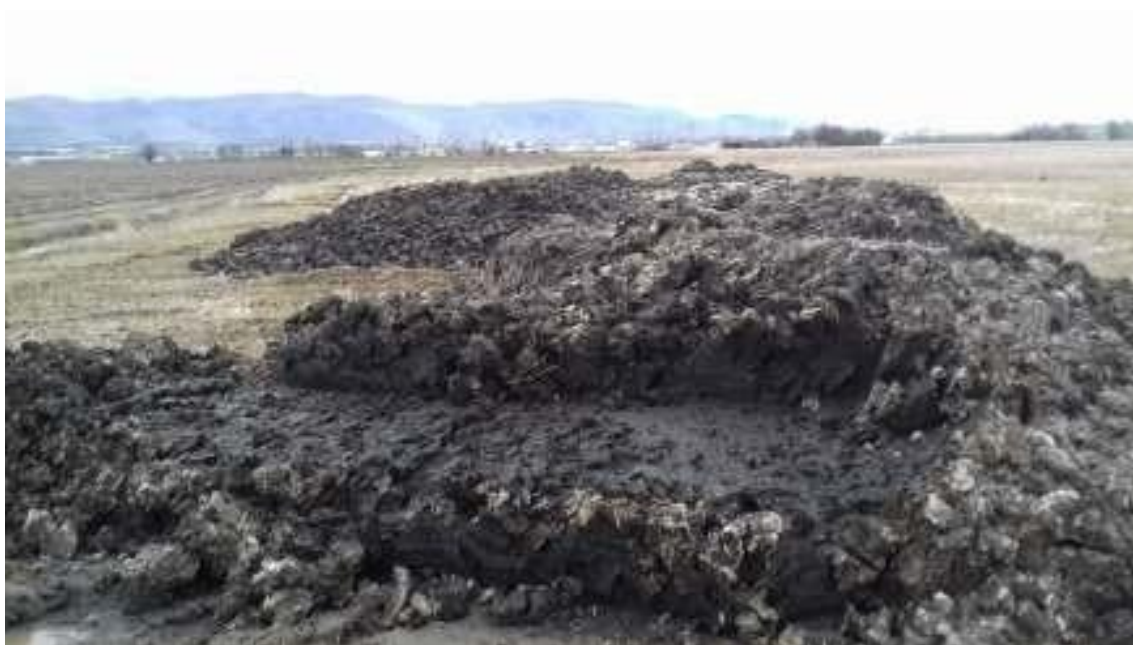
Figure 3 Older lime treated cake prior to hood being placed on cake.
