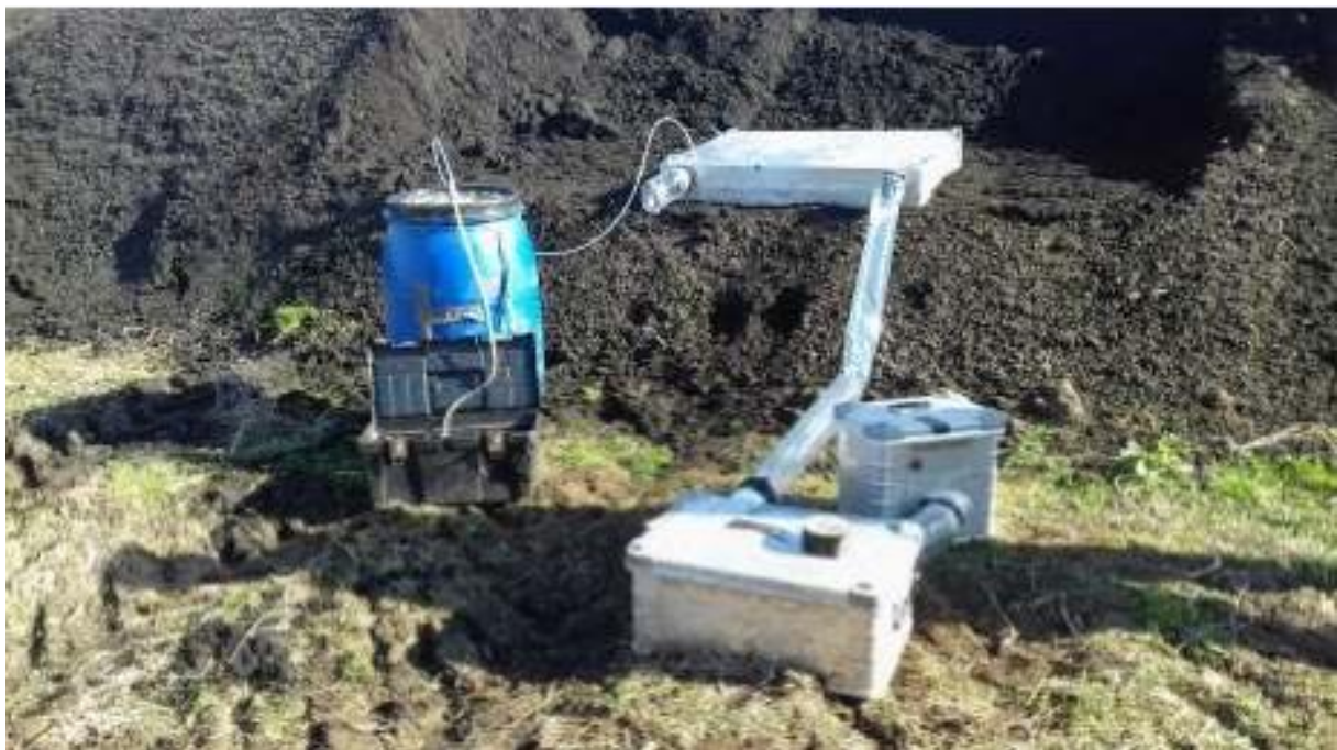
Figure 1 Odour Sampling with Lindvall Hood on relatively ‘friable’ THP digested cake.
