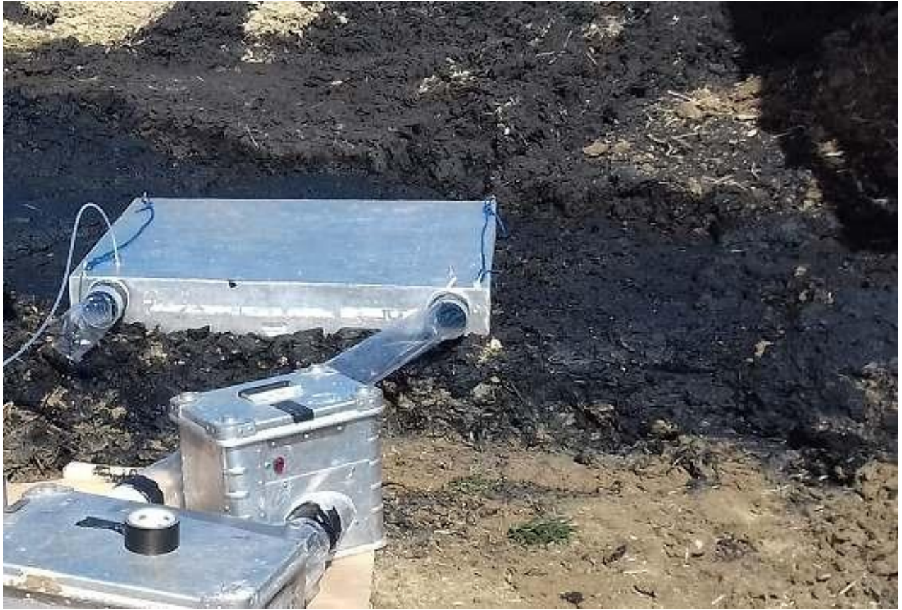
Figure 5 Odour Sampling with Lindvall hood on more ‘fluid’ AD cake.
