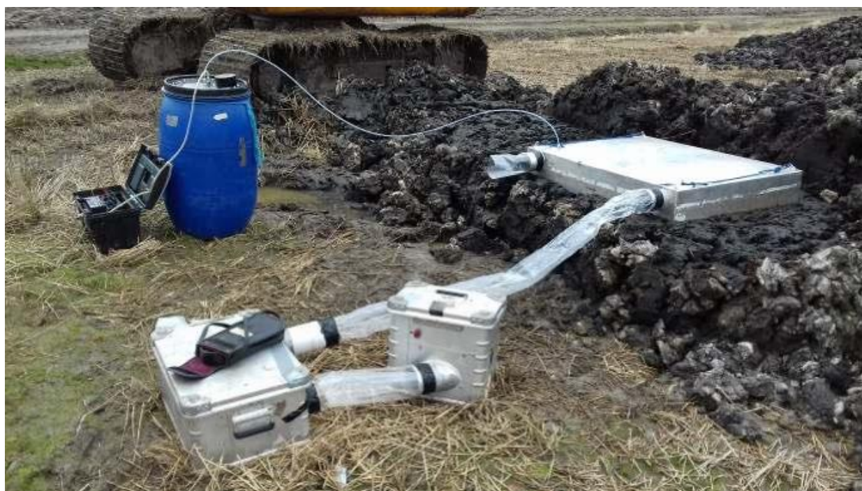
Figure 4 Odour Sampling with Lindvall hood on relatively 'plastic' lime treated cake.
