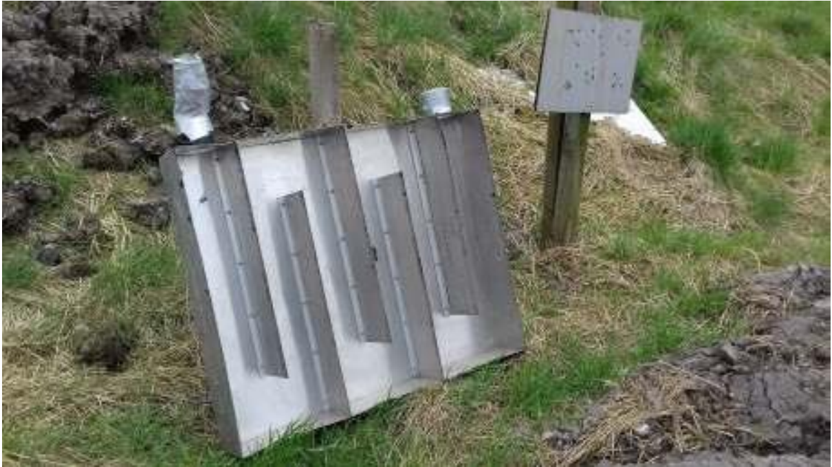
Figure 2 Underside of Lindvall Hood showing internal vanes
