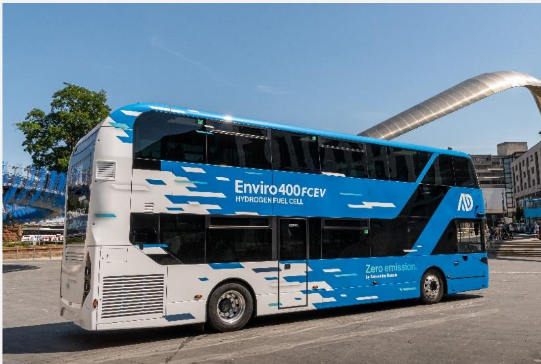
The Enviro400 FCEV – a Hydrogen Fuel Cell Bus Photo Photo credit: Alexander Dennis.
